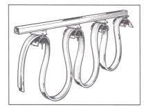
☐ Looped wire festooned bridge electrification systems can include stainless steel suspension cable and non-corroding plastic cable trolleys.
